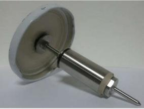
The logger can also be fixed directly to the walls of the package.
