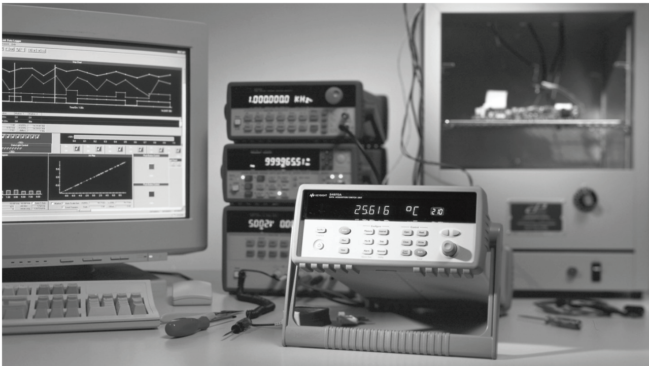
Compact 60-channel data acquisition system
