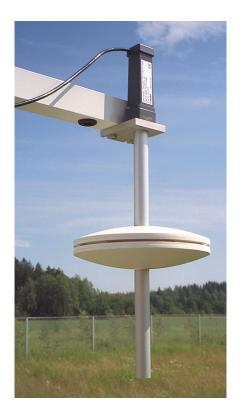
SPH10/20 is easy to install and connect. In the picture, SPH10 is connected to PTB210.
