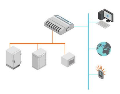
DL1016-1416 data loggers can be used with Vaisala software, either viewLinc or vLog, to download, display, and analyze environmental data.
