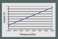
$V_{out}(V) = log (p(hPa)) + 5.5$ p (hPa) =  $10^{(V_{out}(V) - 5.5)}$
