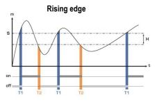
Measurement (m) > Threshold (S) during the time-delay T1  $\rightarrow$  Alarm activation.
