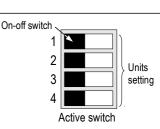
• Configuration by switch : to configure the transmitter, unscrew the 4 screws from the housing then open it.
